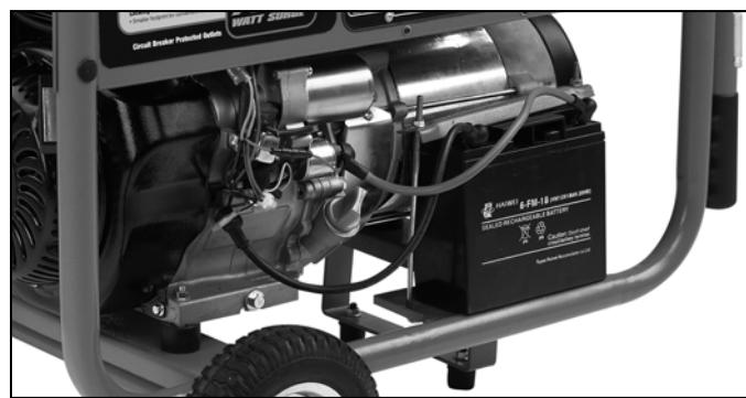
Put the battery on the frame, have the battery assembled with the provided accessories as shown.
